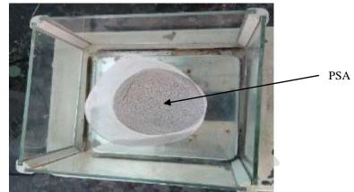
Fig.2: Grinded Periwinkle Shells
