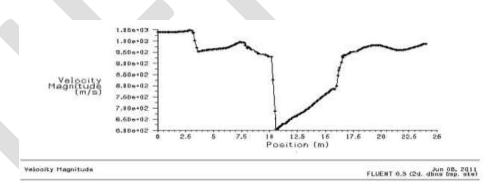
The initial velocity is assumed to be 1050 m/s. According to the contour, in the diffuser section due to the area convergence the velocity is dropped. At the combustion chamber, the velocity remains constant because of the constant area. As the area is diverged at the final in nozzle section, the velocities are raised. Because of the oscillations, velocity raising and dropping are not in expected format. Since, it is due to an unsatisfied condition.
