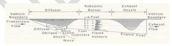
Fig. 1: Two-dimensional Schematic of a Ramjet Engine
