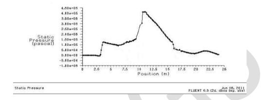
The initial pressure value is assumed to be sea level condition. According to the graph, in the diffuser section due to the area convergence the pressure is raised. At the combustion chamber, the pressure values remains constant because of the constant area. As the area is diverged at the final in nozzle section, the pressure values are dropped. Because of the oscillations, Pressure raising and dropping are not in expected format. Since, it is due to an unsatisfied condition.
