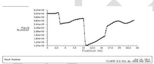
The initial Mach number is assumed to be 3. According to the contour, in the diffuser section due to the area convergence the Mach number is raised. At the combustion chamber, Mach number remains constant because of the constant area. As the area is diverged at the final in nozzle section, the Mach number is dropped.
