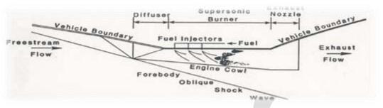
Fig. 2: Two-dimensional Schematic of a Scramjet Engine
