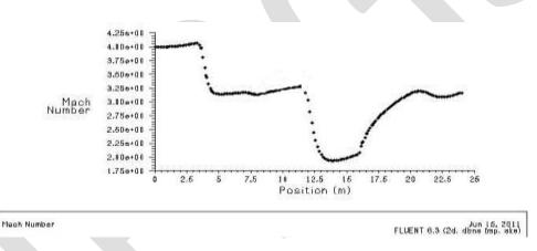
The initial Mach number is assumed to be 4. According to the contour, in the diffuser section due to the area convergence the Mach number is raised. At the combustion chamber, Mach number remains constant because of the constant area. As the area is diverged at the final in nozzle section, the Mach number is dropped.
