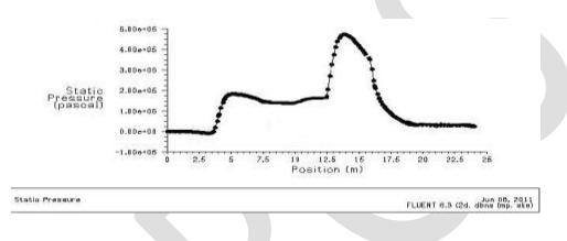
The initial pressure value is assumed to be sea level condition. According to the contour, in the diffuser section due to the area convergence the pressure is raised. At the combustion chamber, the pressure values remains constant because of the constant area. As the area is diverged at the final in nozzle section, the pressure values are dropped.
