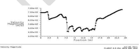
The initial velocity is assumed to be 600 m/s. According to the contour, in the diffuser section due to the area convergence the velocity is dropped. At the combustion chamber, the velocity remains constant because of the constant area. As the area is diverged at the final in nozzle section, the velocities are raised. Because of the oscillations, velocity raising and dropping are not in expected format. Since, it is due to an unsatisfied condition.
