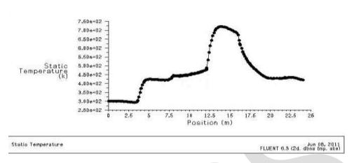
The initial temperature value is assumed to be sea level condition. According to the contour, in the diffuser section due to the pressure raised, temperature value also raised. At the combustion chamber, temperature values remains constant because of the constant pressure. As the final in nozzle section, the temperature values are decreases to decrease the pressure value.
