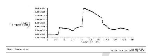
The initial temperature value is assumed to be sea level condition. According to the contour, in the diffuser section due to the pressure raised, temperature value also raised. At the combustion chamber, temperature values remains constant because of the constant pressure. As the final in nozzle section, the temperature values are decreases to decrease the pressure value.
