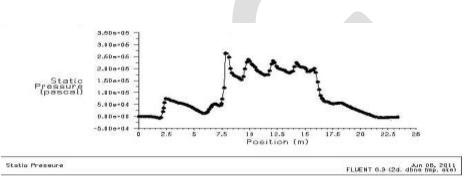
The initial pressure value is assumed to be sea level condition. According to the graph, in the diffuser section due to the area convergence the pressure is raised. At the combustion chamber, the pressure values remains constant because of the constant area. As the area is diverged at the final in nozzle section, the pressure values are dropped. Because of the oscillations, Pressure raising and dropping are not in expected format. Since, it is due to an unsatisfied condition.
