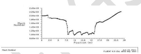
The initial Mach number is assumed to be 2. According to the contour, in the diffuser section due to the area convergence the Mach number is raised. At the combustion chamber, Mach number remains constant because of the constant area. As the area is diverged at the final in nozzle section, the Mach number is dropped.
