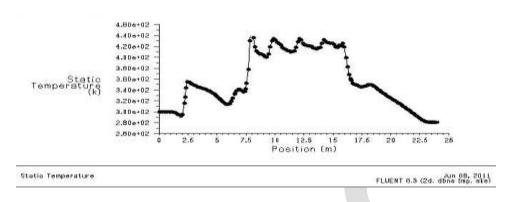
The initial temperature value is assumed to be sea level condition. According to the contour, in the diffuser section due to the pressure raised, temperature value also raised. At the combustion chamber, temperature values remains constant because of the constant pressure. As the final in nozzle section, the temperature values are decreases to decrease the pressure value.
