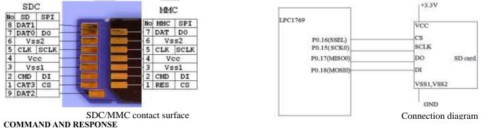
In SPI mode, the data direction on the signal lines are fixed and the data is transferred in byte oriented serial communication. The
