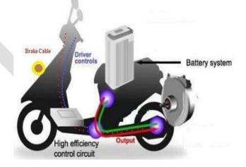
The scooter has a maximum speed of 35km/hr and it is provided with an inbuilt BLDC controller which makes the working of scooter more smooth, silent and efficient.
