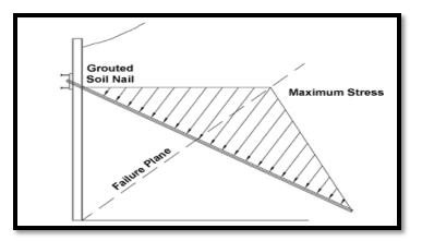
Figure 3: Stress distribution of soil nail
