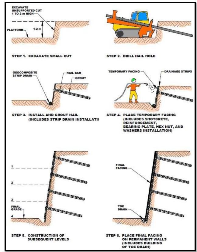
Figure1: Step by step procedure of soil nailing
