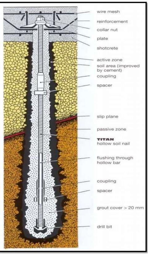
Figure 4: Soil nailing details
