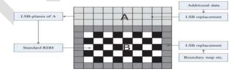
Figure 2. Illustration of image partitioning and embedding process.
