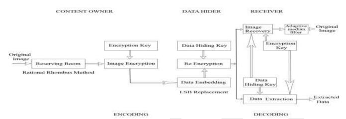
Figure 1. Block diagram of data hiding in encrypted image.
