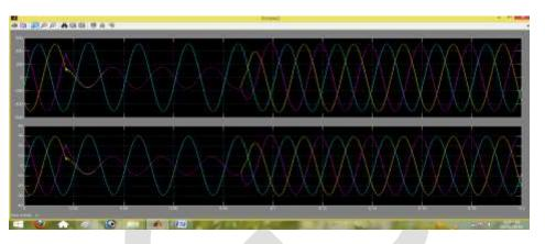
**Figure: 5 Double line-to-ground fault**
