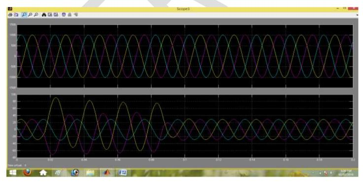
Figure: 7 LL-G Fault waveform of current at input side
