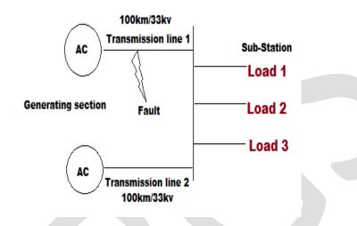
Figure: 1 Show the block diagram of transmission line fault analysis
