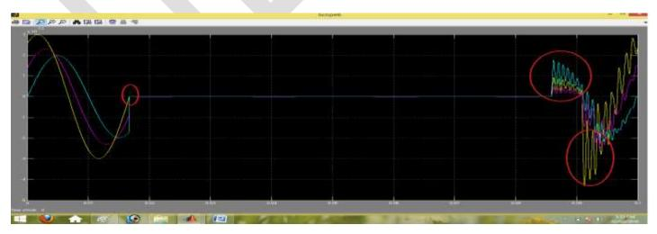
Figure: 12 Fault Current waveform of LLL-G fault Location
