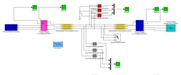
In the above figure-2 three phases Voltage-current (V-I) measurement blocks is used to measure V & I sample at source end. The transmission line is one line 100 Km long. Simulation of three phase fault simulator is used to simulate various types of fault. In transmission line faults are classified as L-G fault, LL-G fault and three phase fault.
