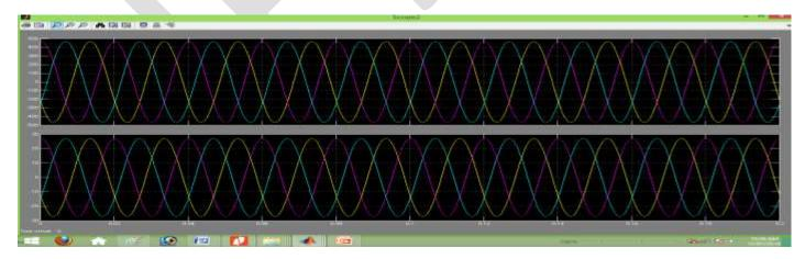
Figure: 9 Voltage and Current waveform of healthy network
