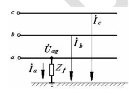
Figure: 3 Single line-to-ground fault
