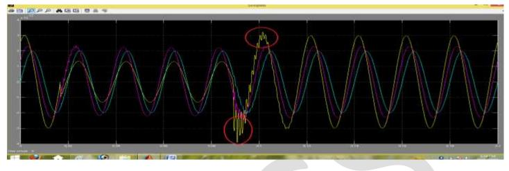
Figure: 10 Fault Current waveform of L-G fault location
