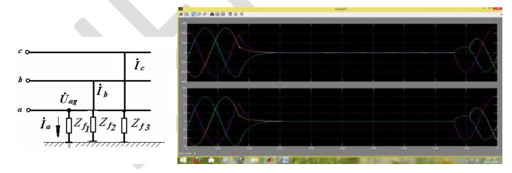
Figure: 7 Triple line-to-ground fault
