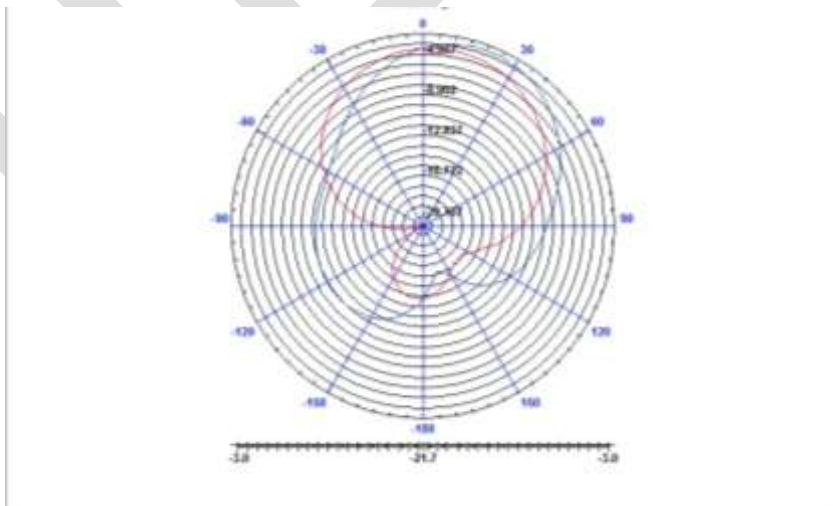
Figure 7 radiation pattern 1x2 inverted diamond array with T slot
