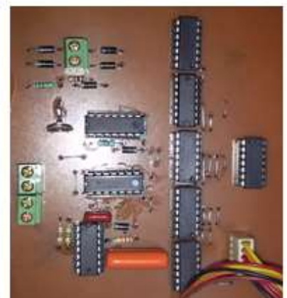
Figure 9 Actual PCB of Control circuit
