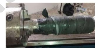
Fig 3: Tube strip wound on mandrel
