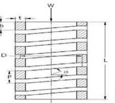
Fig 1: Spring with rectangular cross-section
