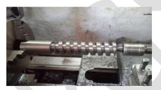
Fig 2: Helical groove cutting process.
