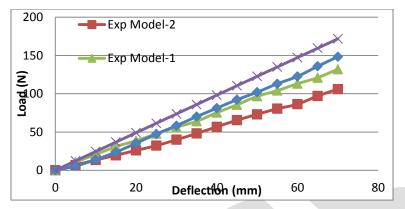
Fig 6: Load- deflection plots for Theoretical and Experimental spring models
