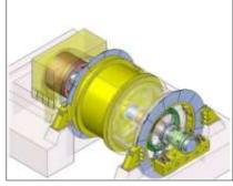
Fig.:- Closed Disc drum
