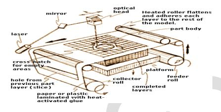
Material is usually a paper sheet laminated with adhesive on one side, but plastic and metal laminates are appearing.
