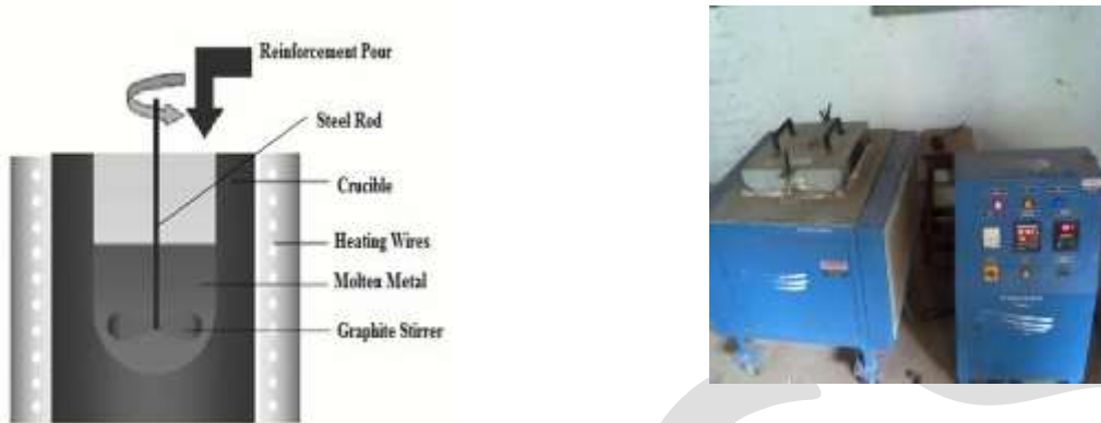
Fig 1: shows the graphical representation of Stir casting and Resistance Furnace
