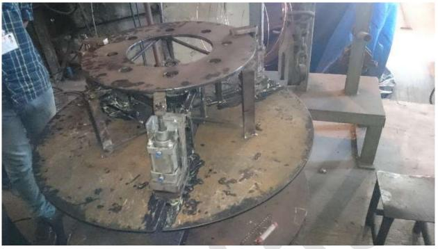
Figure 7. Self-Centering Mechanism with plate
