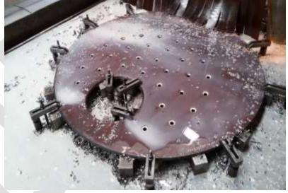
Figure 1. Actual Mounting of Plate
