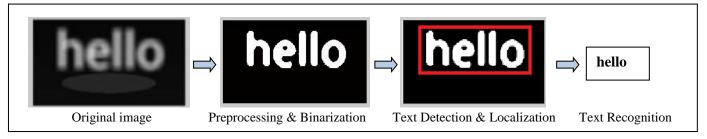
Figure 6: Text Extraction process on image
