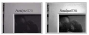
Figure 4: Contrast Enhancement using Histogram equalization.
