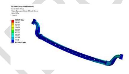
Figure.7. Von mises stress distribution for W<sub>1</sub>and W<sub>2</sub>
