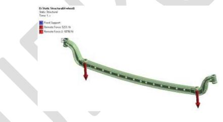
Figure.4. Boundary conditions due to gyroscopic effect
