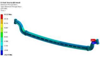
Figure.8. Maximum principal stress distribution for W1and W2
