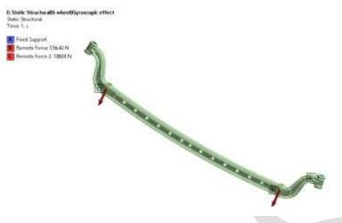
Figure.3. Boundary conditions due to gyroscopic effect
