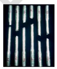
Figure 3. Specimens which undergone Tensile Test.
