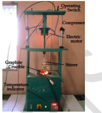
Figure 1. Stir Casting setup for fabrication of (Al8011/ B<sub>4</sub>C/ Red Mud)
