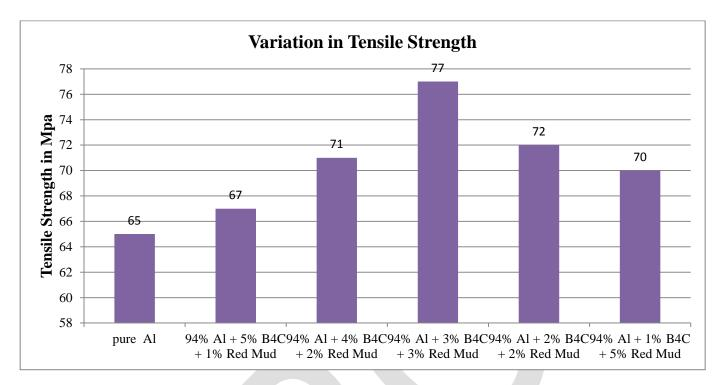
Fig.9 graph shows the variation in tensile strength from 5-1% of B₄C and 1-5% Red mud composite
