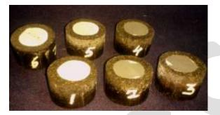
Figure 4. Prepared specimens for Vickers Hardness Test
