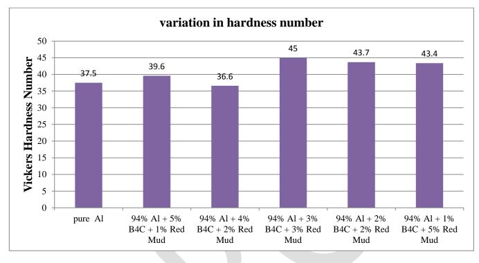
Fig.11 graph shows the variation in Hardness Number from 5-1% of B<sub>4</sub>C and 1-5% Red mud composite
