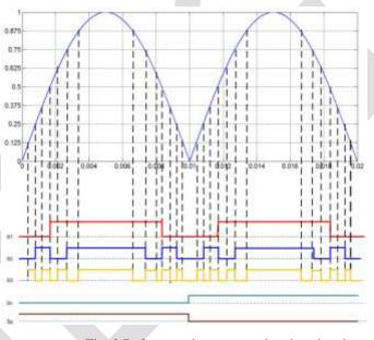
Fig. 3:Reference sine wave and gating signals.
