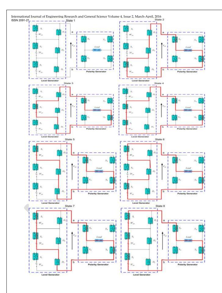
Fig.4: Operating states of the proposed inverter.
