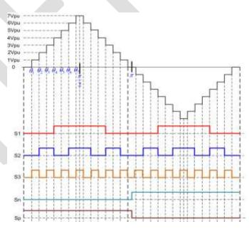
State 3:  $V_{ab} = 50V$  -To obtain this state of level 2 switches S2, SP are ON and remaining switches are OFF.
