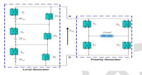
Fig. 1:Proposed asymmetrical 15-level inverter topology.
