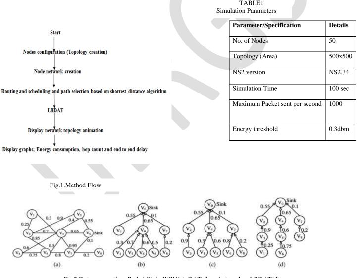
Fig.2.Data aggregation: Probabilistic WSN(a), DATs(b and c), and an LBDAT(d)
