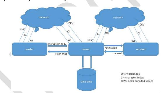
Message entered by user is encrypted at client side and then ciphered text is sent to server and stored on to the server. Server store encrypted message in message data base and then notify appropriate receiver about message. Whenever receiver login into the system and request for the message, server sent ciphered values to the receiver and decryption take place at the receiver end. Then original message will be sent to receivers email address.
