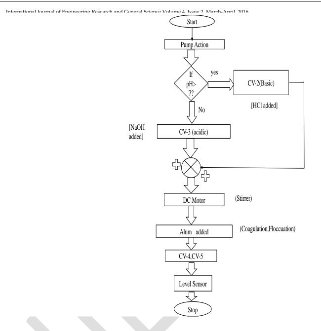
Fig.9 Flow Diagram of Process
