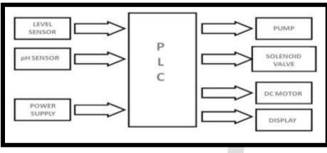
Fig.1 Block Diagram of PLC based ETP
