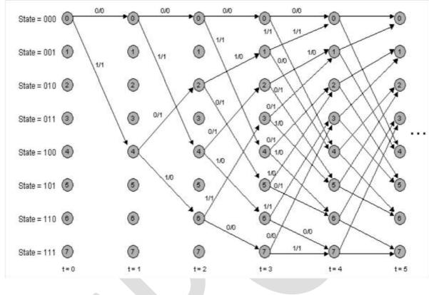
Fig 10: Trellis Diagram for one 8 State Constituent Encoder [8]
