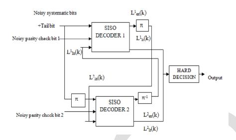
Fig 8: Structure of a Turbo Decoder based on either SOVA or the BCJR Algorithm [8]
