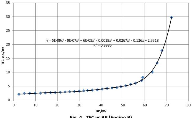
Fig. 4, TFC vs BP (Engine B)
