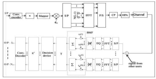
Fig.9. MC-CDMA internal block diagram
