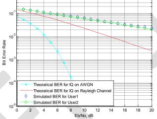
Fig.14.BER Vs Eb/No using Gold code.
