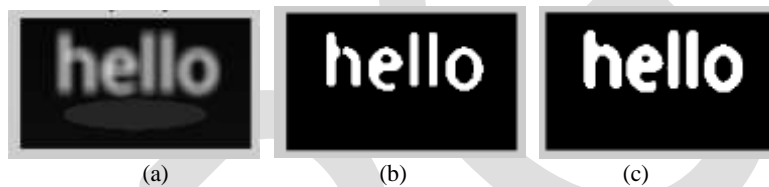
Figure 2: De-blurring of an image using Wiener filter. (a) Blurred image; (b) Binarized image without filtering; (c) Binarization after De-blurring
