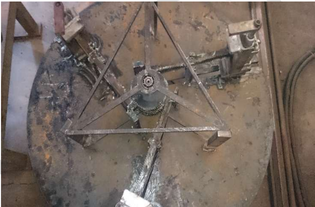
Figure 6. Self-Centering Mechanism without plate
