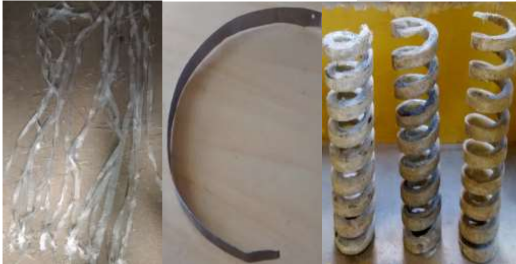
Fig 4: Fiber and steel strip with 90° orientations
