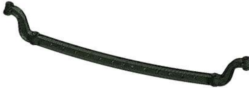
Figure.5.Finite element model of Front axle beam
