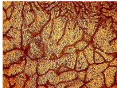
Figure 6. Pure Al without reinforcements
