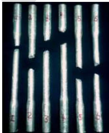
Figure 3. Specimens which undergone Tensile Test.
