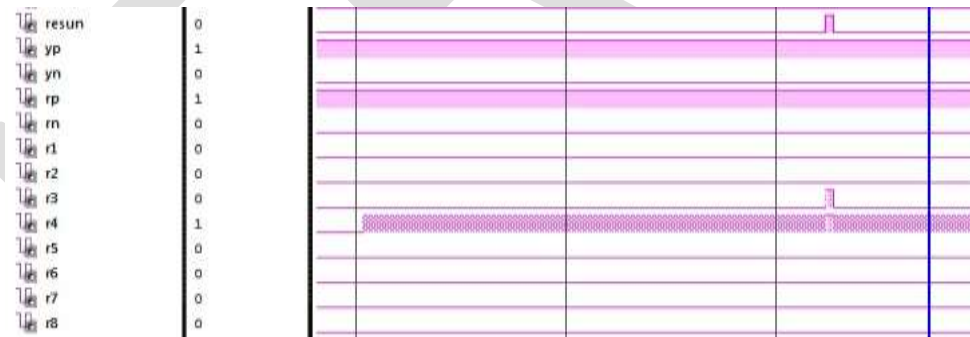
Fig 8. Simulation waveform of thruster selection logic
