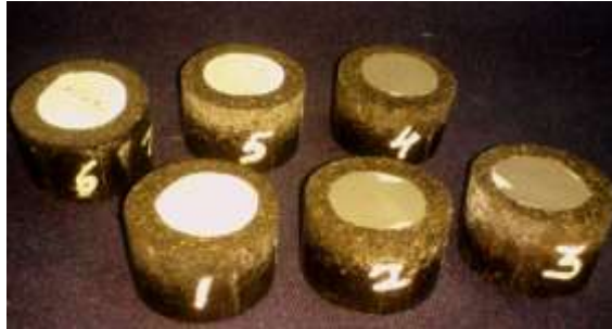
Figure 4. Prepared specimens for Vickers Hardness Test
