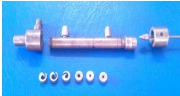
Fig. 2: Parts of Vortex Tube used for experiments
