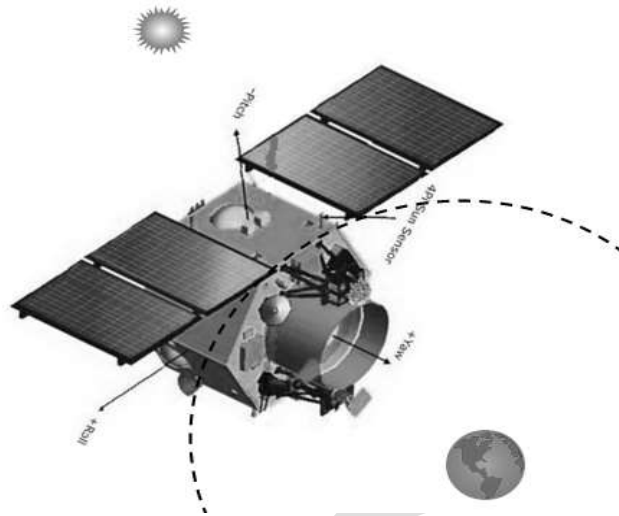
Fig 1. Satellite's position w.r.t.to the Earth and the Sun
