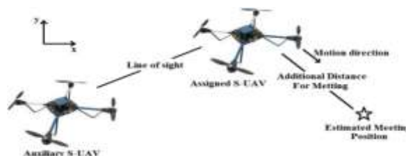
Figure 3: PN method for tracking of the assigned S-UAV
