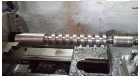
Fig 2: Helical groove cutting process.
