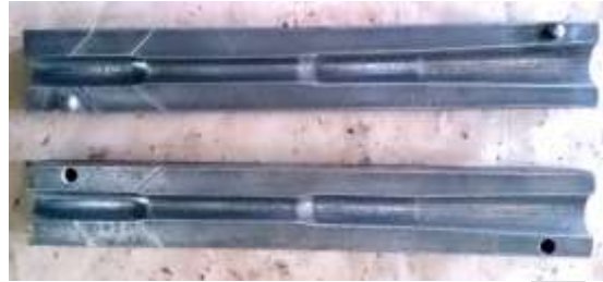
Figure 2. Die used for Stir Casting
