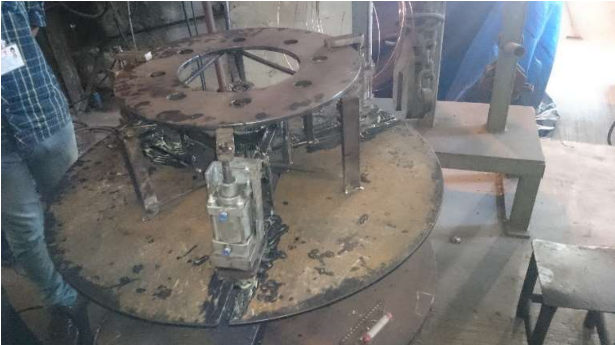
Figure 7. Self-Centering Mechanism with plate
