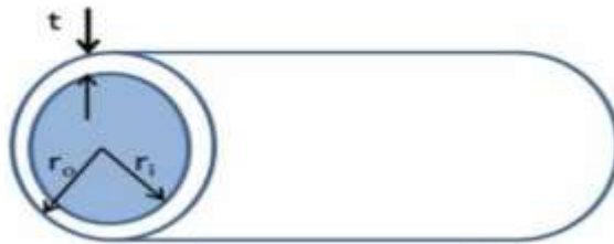
Figure 3: Dimensions of cylindrical pipe.
