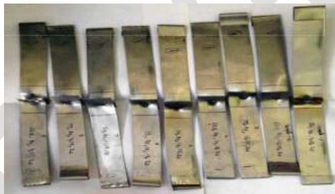
Fig 1: Test specimens after tensile testing on UTM m/c
