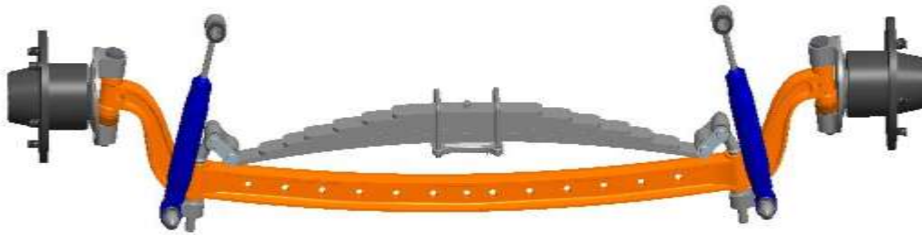
Figure.1. Dead Front Axle Mechanism of Commercial Truck
