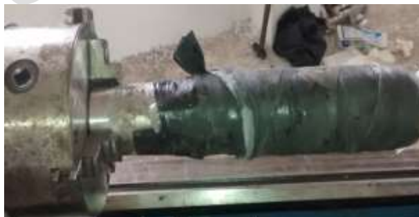
Fig 3: Tube strip wound on mandrel
