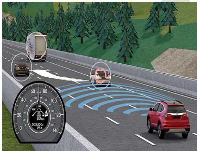
Figure 1. Adaptive Cruise Control using Radar based systems
