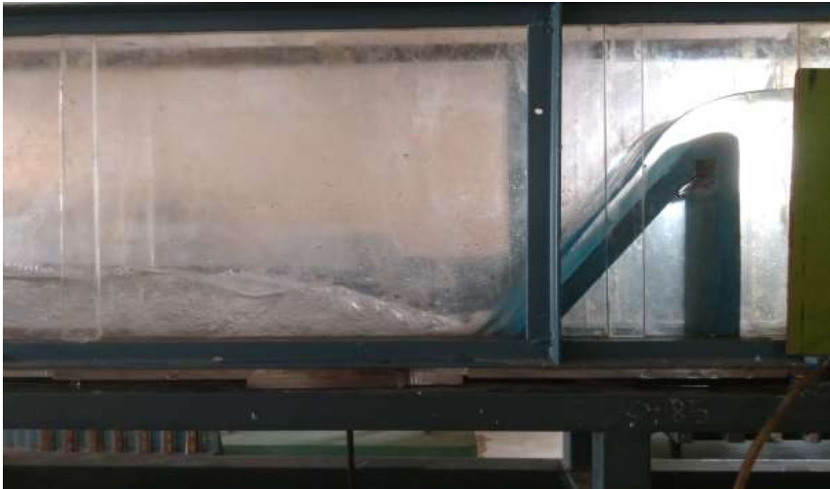
Fig.2 hydraulic jump at the toe of spillway
