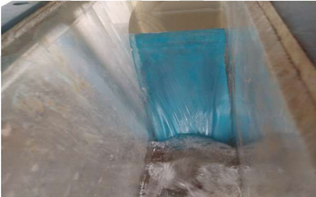
Fig.1 flow over ogee spillway
