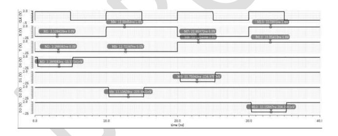
Fig 5: Transient analysis for dynamic NAND 2:4 decoder with four stage CMOS taper bypass buffer
