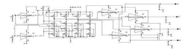
Fig 2: Integration of Dynamic NAND 2:4 decoder with conventional four stage taper buffer circuit
