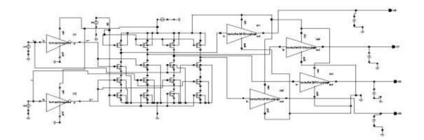
Fig 4: Integration of dynamic NAND 2:4 decoder with four stage CMOS taper with bypass buffer
