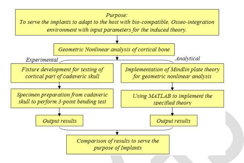
Figure 1: Overall procedure for the Non-linear analysis of cortical bone
