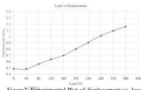
Figure7: Experimental Plot of displacement vs. load
