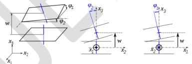
Figure 2: Out of plane deformation according to Mindlin plate theory.
