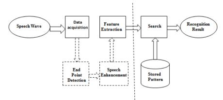
Fig.1. Block diagram for Speech Recognition
