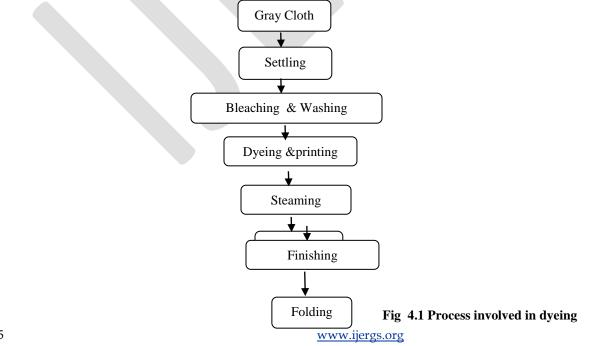
Dyeing methods have not changed much with time. Basically water is used to clean, dyeand apply auxiliary chemicals to the fabrics, and also to rinse the treated fibers or fabrics.
