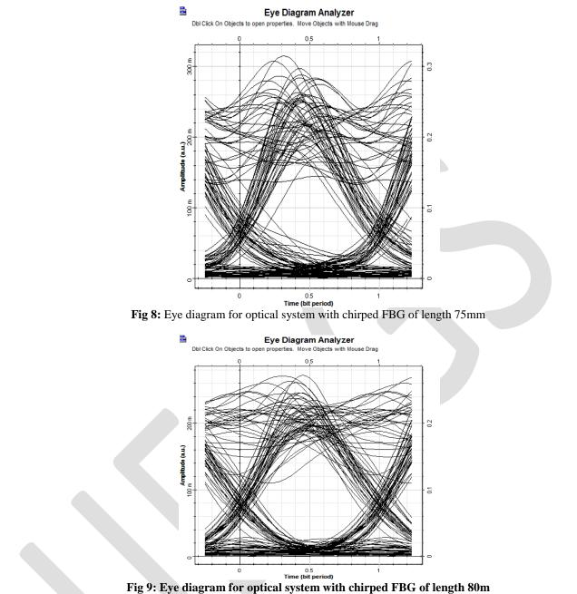
From the above three eye patterns for different lengths of FBG as the length increase the better the eye opening and interference is also less. So the Q-factor is increases and the bit error rate is decreases.
