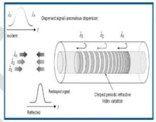
Fig2: A chirped FBG principle
