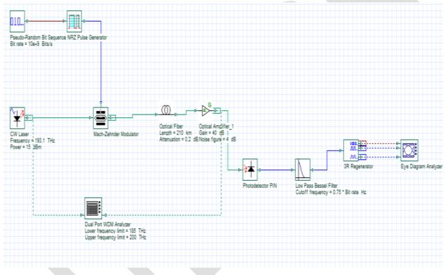
Fig 3: Model of Simulation using OptiSystem
