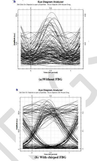
Fig 10: Comparison of eye diagrams
