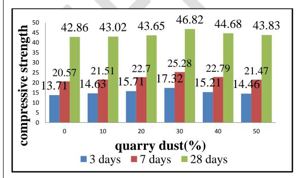
• Examining the strength at 28 days age it can be seen that increasing the quarry dust content from 0% to 20 % has caused increase in compressive strength by 2% as compared to reference mix.
