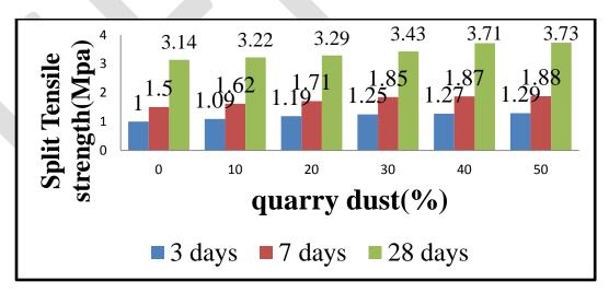
• It is clear that the splitting-tensile strengths of quarry dust SCC mixtures are increasing. The increase was almost 8% at 30% partial replacement while it was almost 15% at about 40% partial replacement.
