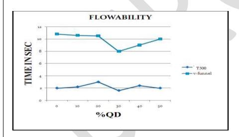
At 30% Partial replacement of fine aggregate by quarry dust the time of flow in slump flow test and in V Funnel test was observed to be minimum.
