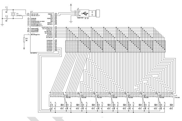
Figure 5: Circuit Diagram for A GSM Based Scrolling LED Display System
