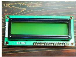
Fig 10: Liquid Crystal Display
