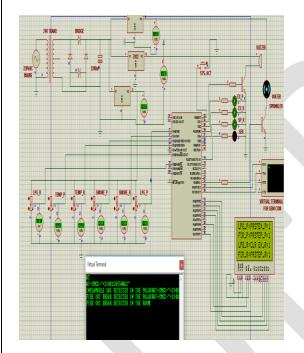
Fig 15: simulated result when there is presence of gas in the parlor, present of fire in the parlor and room.
