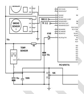
Fig 5: circuit of interfacing lm35 sensor
