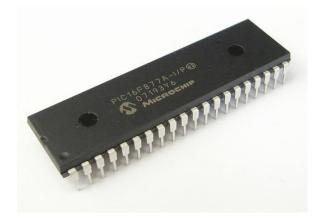
Fig 6: PIC16F877A Microcontroller
