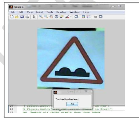
Fig V: Results of detection of traffic sign board
