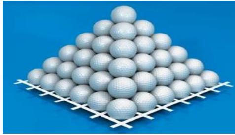
Fig. 1 Representation of geogrid confining the aggregates
