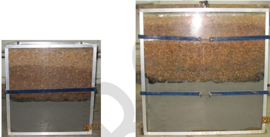
Fig. 2. Model of soil sample prepared for consolidation test
