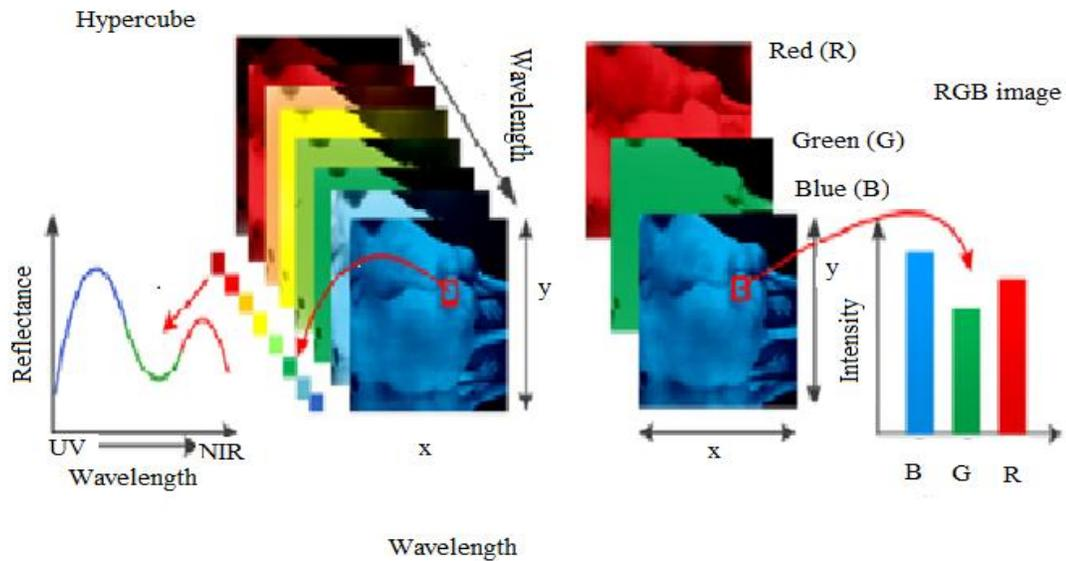
Fig1: Comparison between hypercube and RGB image
