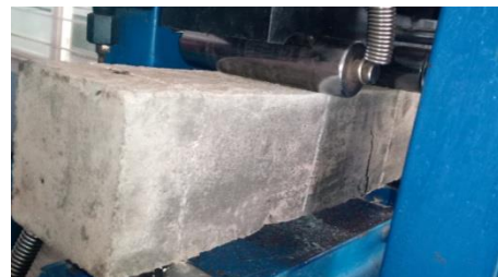
Fig. 5 Failure of Beam with PET mesh
