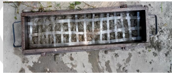
Fig. 3 Placing of mesh during casting
