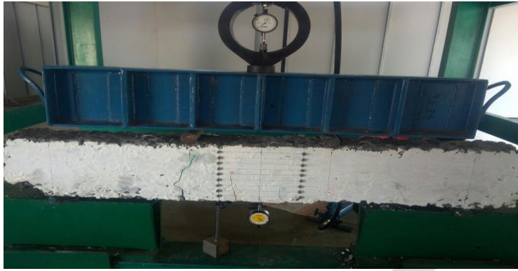
Fig. 3 Failure of beam with treated PALF
