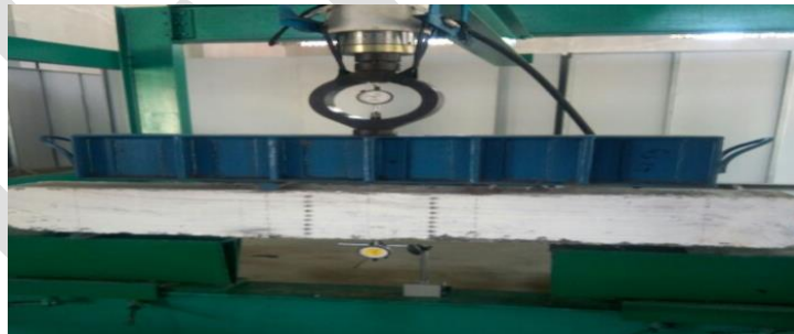
Fig. 2 Failure of control beam
