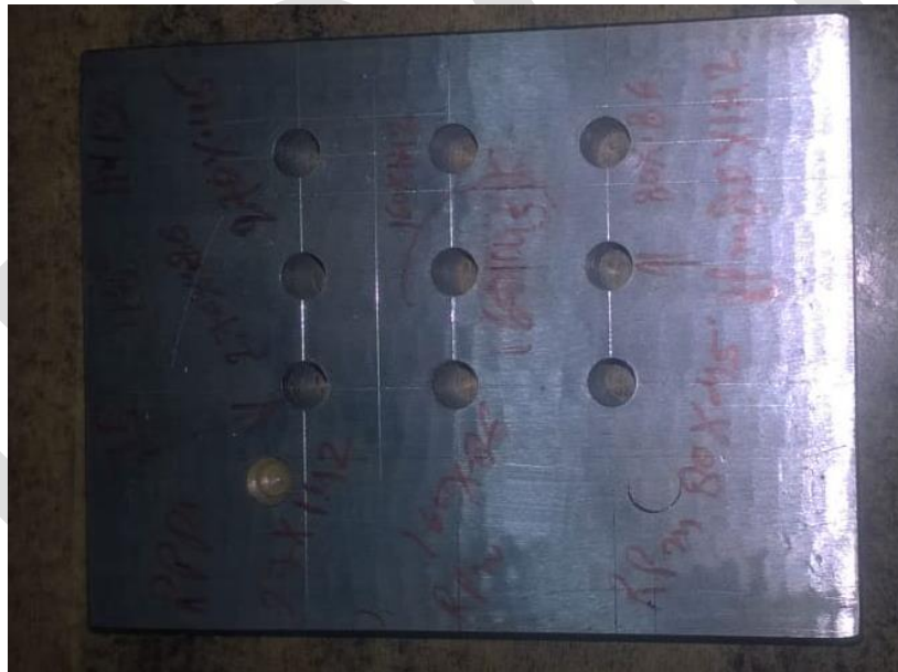
Figure: 1. Mild Steel work piece after Drilling
