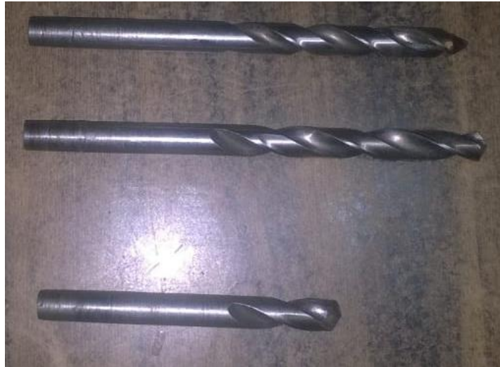
Figure: 2. Different point angle HSS Drill Bit
