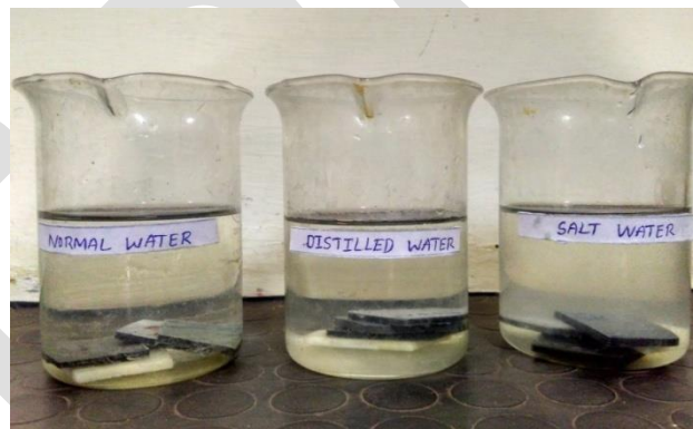
Fig. 4. Test specimens immersed in normal, distilled and salt water
