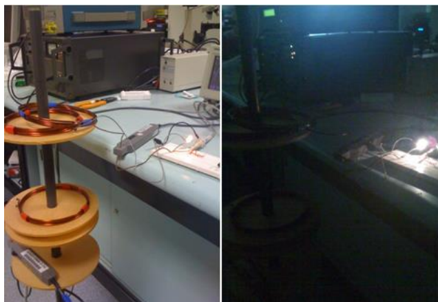
Fig. 10: Bulbs of different rating lit wirelessly with high efficiencies.
