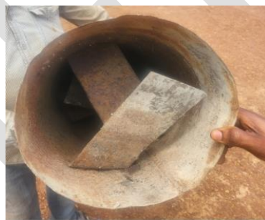
(b) Welded blades/fractionating columns
