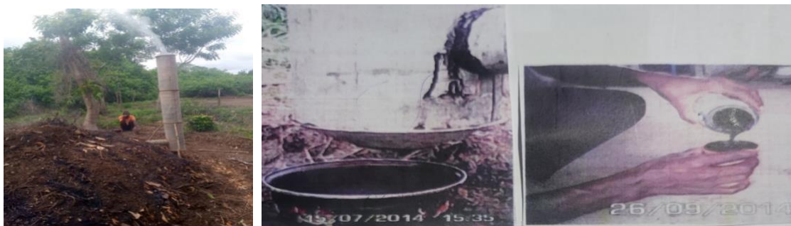
1. Pyrolysis in progress (b) Condensation of tar from chimney (c) Measuring tar collected
