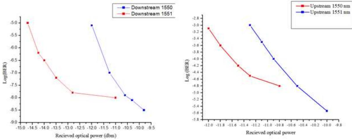
Fig. 5. Transmission performance of downstream and Upstream data
