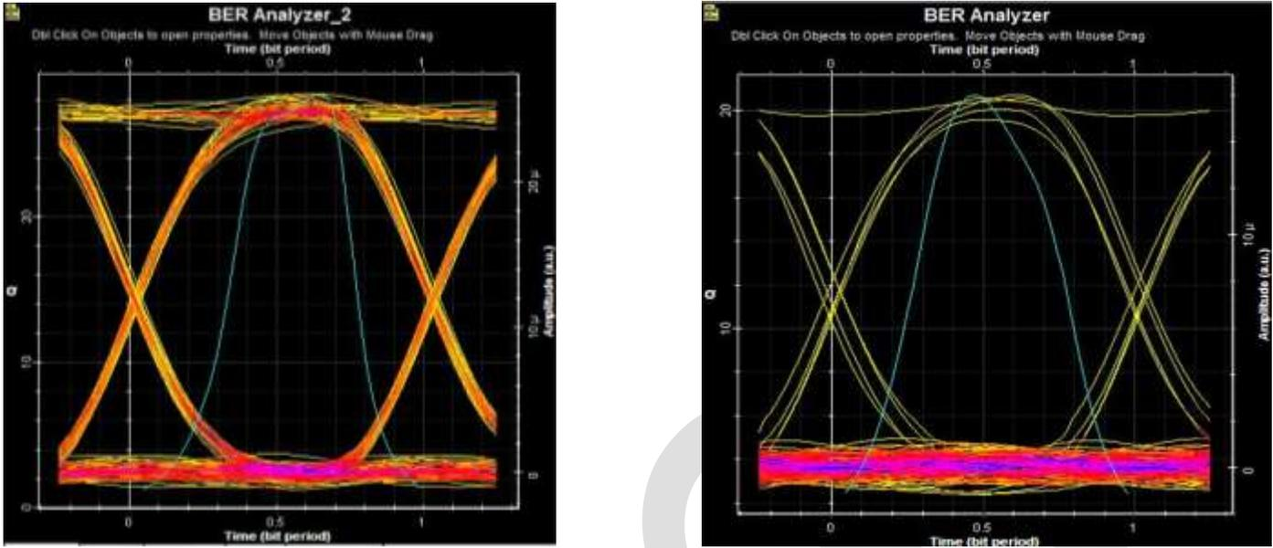
FIG. 4. EYE DIAGRAM FOR (A).DOWNSTREAM AND (B) UPSTREAM SIGNAL
