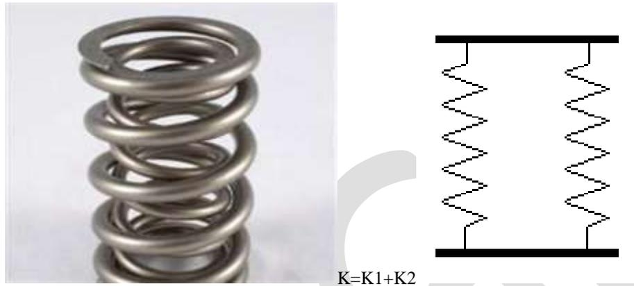
Figure1: Helical compression springs in pallel.
