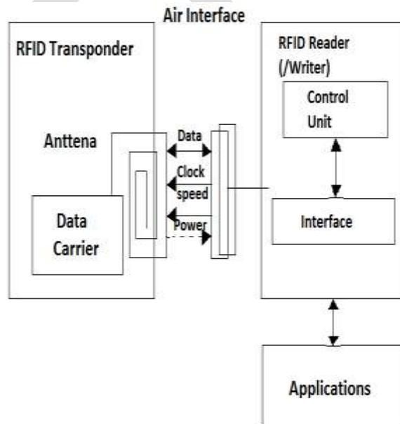
Fig2: RFID working principle
