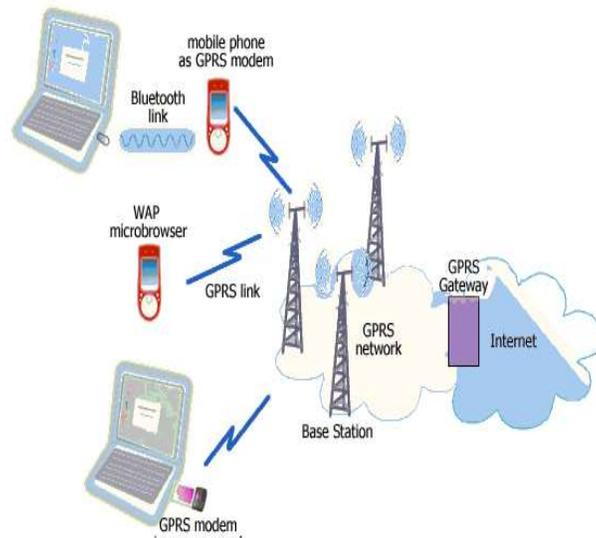
*Fig5: GPRS Structure*
