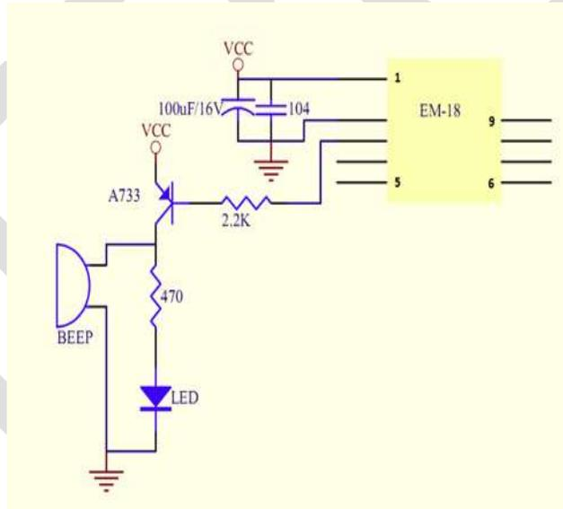
*Fig4: EM-18 Application Circuit*
