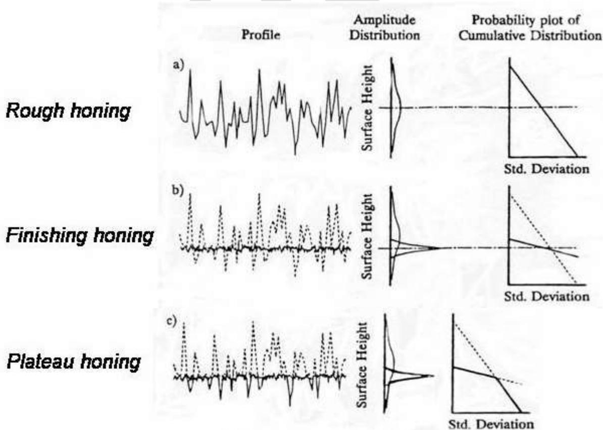
**Figure 4. Combination of processes of honing.**
