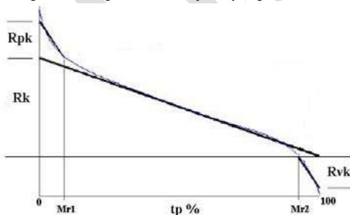
Figure 2. Abbott-Firestone Curve and parameters.
