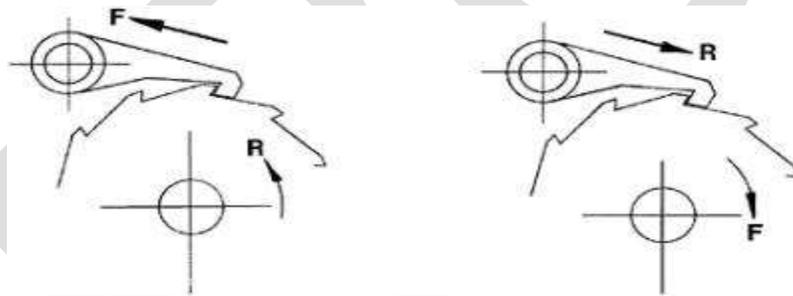
Figure 3: Variation of ratchet and pawl action ( $F$  = force;  $R$  = reaction).
