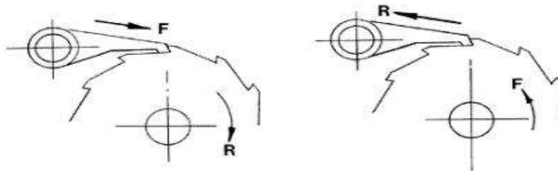
Figure 2: Variation of ratchet and pawl action ( $F$  = force;  $R$  = reaction).
