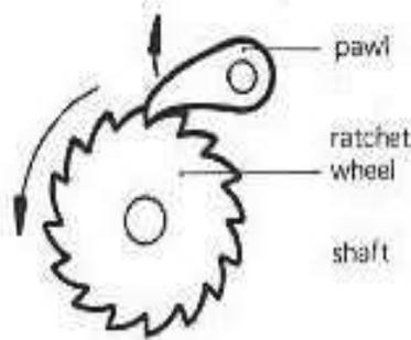
Fig.4.Ratchet pawl mechanism
