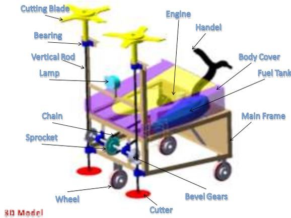
**Fig 4: 3D Model of Sugarcane Harvesting Machine**
