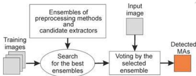
Figure 4 : Flow chart of the ensemble-based framework.
